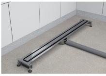
2. The adjustable legs (optional additional payment) should be glued in the places shown. Connect the channel to the drainage system and set the height using the adjustable legs so that the upper edge of the frame is approximately 1mm below the the finished surface level of the shower. We recommend that you do not remove the protective foil from the grating until the installation is complete.
