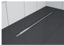
8. Once the liquid foil is completely dry as per the manufacturer's instructions, the shower surface can be tiled (eg ceramic tiles or granite). Seal the gap between the tiles and the channel frame with flexible sanitary silicone compatible with the tile and grout colour.
