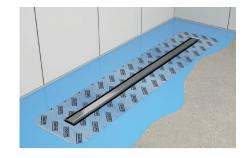
5. Apply the sealing membrane (optional additional payment) in position on the in position on the freshly applied liquid foil.
