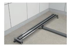
2. Connect the channel to the drainage system and set the height using the adjustable legs so that the upper edge of the frame is approximately 1mm below the finished surface level of the shower.
