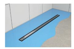
4. Cover the flange and the surrouding area with an insulating foil in a liquid form.
