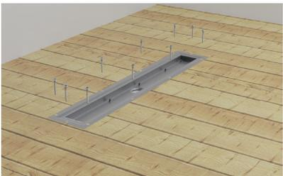
3. Connect the channel to the drainage system. Make sure that linear drain is flushed in the wooden floor. It is absolutely necessary to remember about the appropriate slope in the wooden floor, which must be at least 2%.
