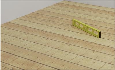
1. Set the level of the finished shower floor surface and establish future shower area by placing the linear drain on top of existing floor boards. Use pencil to draw perimeter around the drain outlet to mark the position of the linear drain and waste trap.
